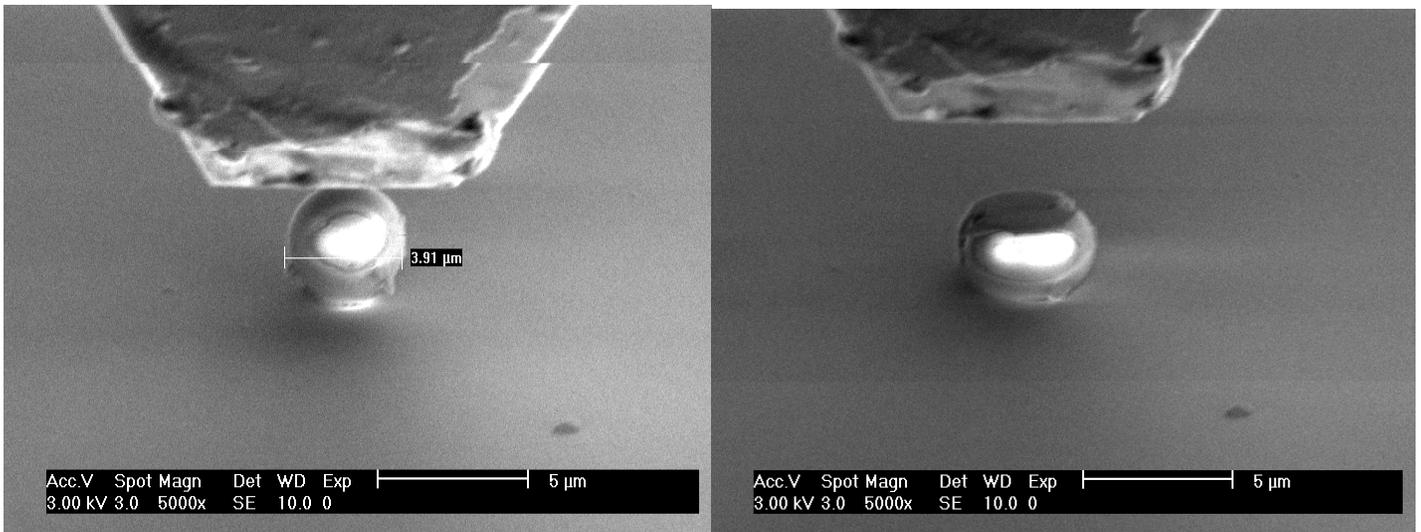
**Figure 3** – Microsphere before and after testing: (a) Before testing; (b) After plastic yielding and fracture.
