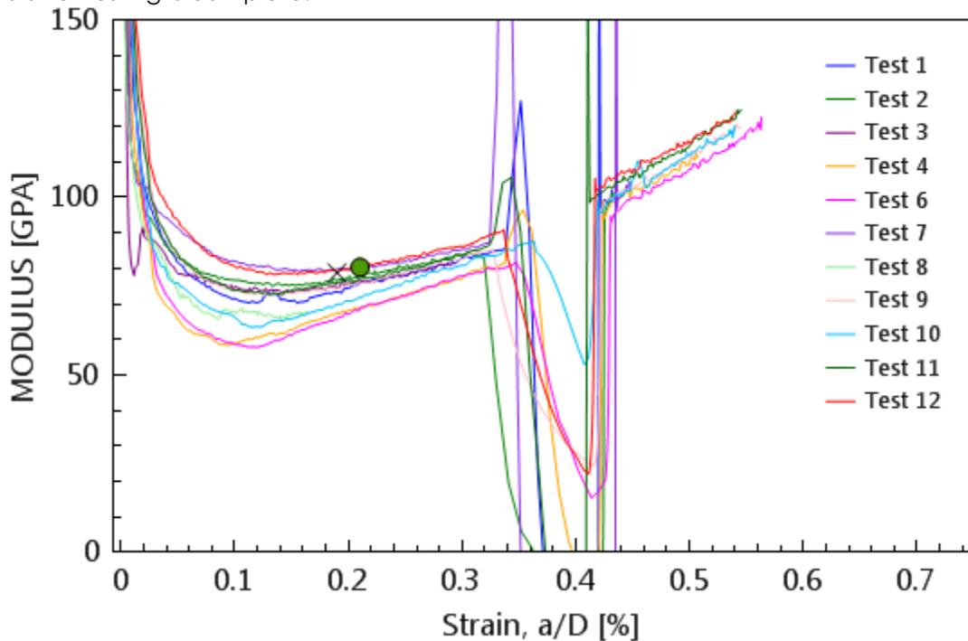
**Figure 4** - Modulus as a function of compressive strain for twelve microspheres. Failure is obvious at strains just greater than 0.3%.
